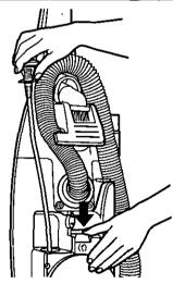
2) To rewind the power supply cord, press and hold the rewind button, allowing the power supply cord to be automatically rewound into the cleaner.
